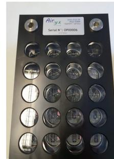
Retro reflector array to be placed at the end of the measurement path to reflect light back to telescope. Water proof IP67 housing with changeable desiccant.
