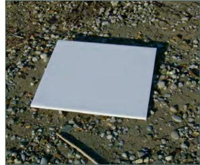
*Zenith Alucore targets withstand harsh environmental conditions such as UV radiation, rain and snow without losing their reflective and high lambertian properties.*
