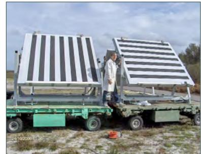
*Positioned at the end of runways, multi-step Alucore targets can be used to help pilots adjust and calibrate their measurement equipment.*
